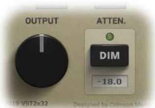
Output knob controls the master output volume.
