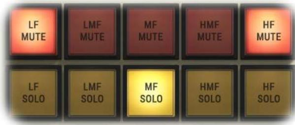
10 buttons to solo or mute the 5 frequency bands. Solo buttons override mute buttons. Click with shift left mouse button on any button deactivates all other buttons. This helps to quickly click through individual bands.
