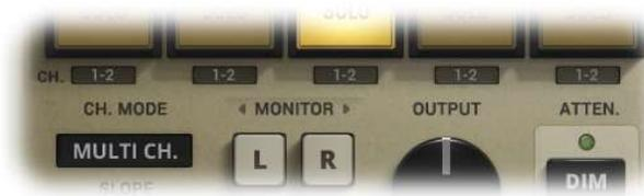
If “Ch. Mode” is set to **multi channel**, ISOL8 copies the split band to one out of five channel pairs/buses.
