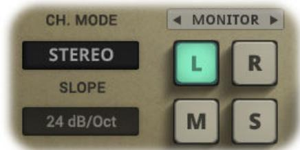
Channel mode will apply the filter only to the selected channel: Stereo, Left, Right, Mid/Sum or Side/Diff signal.
