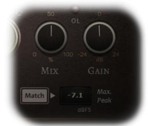
The gain control adjusts the output volume. The small LED above the process knob indicates signal clipping (> 0.0 dBFS).
