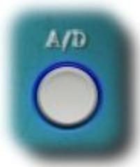
"A/D" - button switches between analog and digital filtering. Lighted button means "A" or analog filter. This button is only relevant during "processing" - state.
