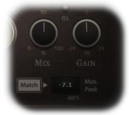
The gain control adjusts the output volume. The small LED above the process knob indicates signal clipping (> 0.0 dBFS).
